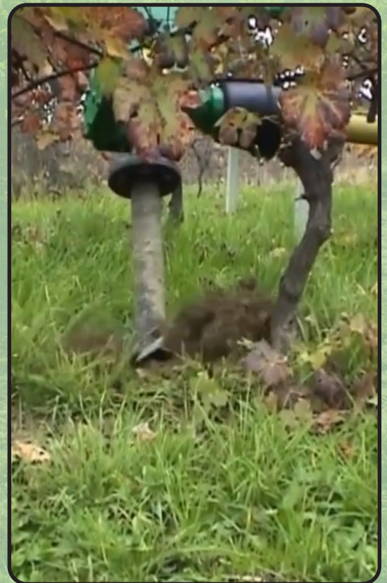
Working Arm Lateral Stroke: 34" Central Position Stroke: 47" Total Length: 83" Total Width: 36"
