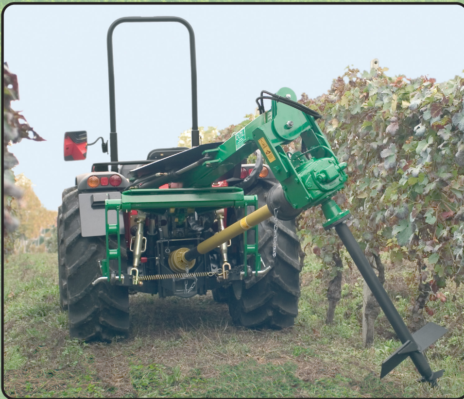
Working Arm Lateral Stroke: 34" Central Position Stroke: 47" Total Length: 83" Total Width: 36"
